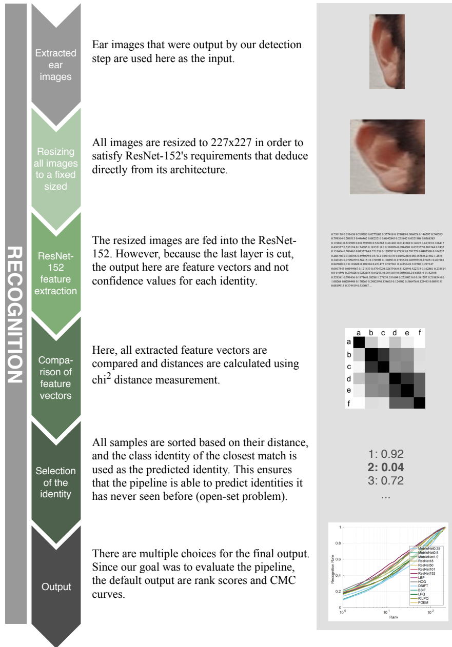
Fig. 3: A diagram of the unified pipeline. The detection part of the pipeline (in blue) is assembled mainly from RefineNet detector and the recognition part of the pipeline (in green) is assembled mainly from ResNet-152. The inputs are arbitrary images of subjects, the outputs are the subjects' identities.
