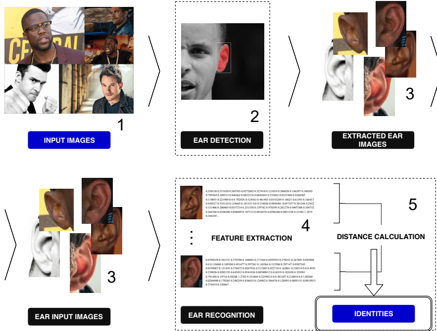
Fig. 1: Diagram of the proposed unified ear recognition pipeline. The inputs are arbitrary images of subjects (1), the output of the pipeline are identities based only on ear biometrics (5). Ear detection (2) is performed on images of subjects, which outputs cropped ear images (3) that serve as the input into ear recognition step (4 and 5).
